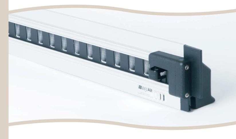
Passive background ventilation takes advantage of the varying air pressure that wind creates around a building. On the windiest side, positive air pressure pushes fresh, dry air inside through the Easy Air vents. Negative air pressure then draws damp stale air out of the home on the sheltered side. All that is required is one vent in each room.
